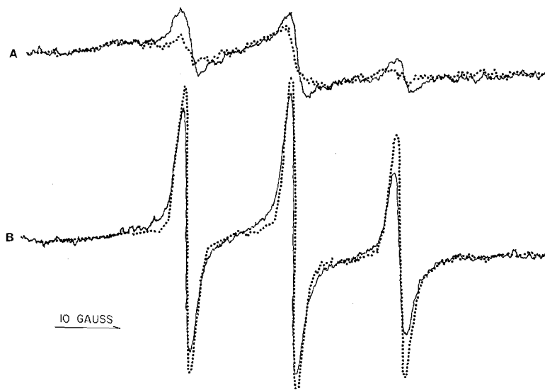
Figure 1. Electron spin resonance spectra of N-(1-oxyl-2,2,6,6-tetramethyl-4-piperidinyl) bromoacetamide covalently bonded to H. salinarium cell envelope. (A) Dotted line (.....): Resonance spectrum in 4 M NaCl. Solid line (—): Resonance spectrum in 4 M NaCl after exposure to distilled water (compare to (B) solid line spectrum). (B) Solid line (—): Resonance spectrum in distilled water. Dotted line (.....): Resonance spectrum in distilled water after treatment with trypsin (1 mg/ml) for 15-30 min. All resonance spectra were recorded at identical instrument setting.
